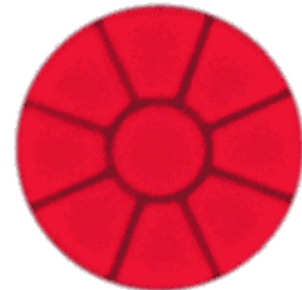
collimated far field beam pattern target distance = 7.2 m dot diameter = 78 mm
