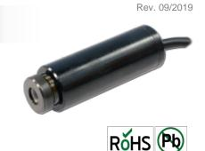
**RLDD405** series of Diode Laser Modules has been designed with emphasis on *superior beam quality*, and *reliable operation*. The modules body is made of black anodized aluminum, enclosing laser diode, lens, and driving electronics. RLDD405 series features a *focusable glass lens optic* with a locking mechanism. The supply voltage is specified with *3 VDC*.
