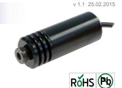
**RLDH850** series of Diode Laser Modules has been designed with emphasis on *superior beam quality*, and *reliable operation*. The modules body is made of black anodized aluminum, enclosing laser diode, lens, and driving electronics. RLH850 series features a *focusable glass lens optic* with a locking mechanism. The supply voltage is specified with *3 VDC*.
