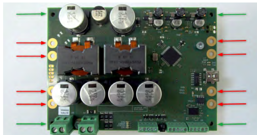
Fig. 3: Mounting holes (green arrows) - Contact pads (red arrows)
