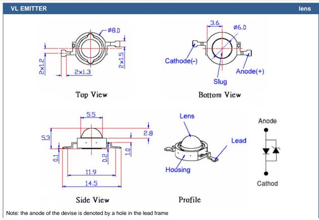
All Dimensions in mm; Tolerance: ±0.2 mm
