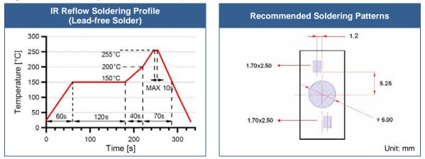
Above table specifies the maximum allowed duration and temperature during soldering. It is strongly advised to perform soldering at the shortest time and lowest temperature possible.
