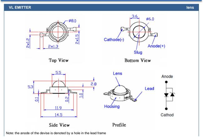
All Dimensions in mm; Tolerance: ±0.2 mm
